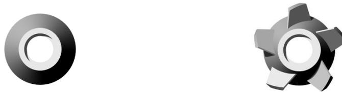
Figure 5- Hi-Fin model, left: Base case, right: Hi-Fin
